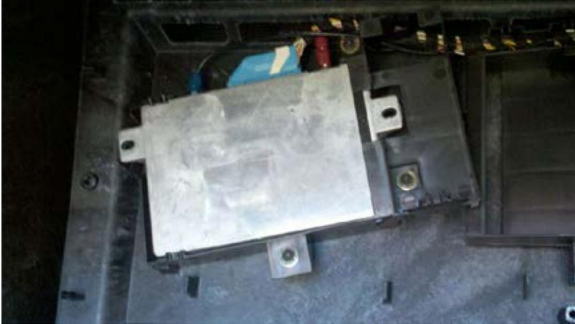
*2004 Phaeton OnStar controller mounted on equipment shelf*
