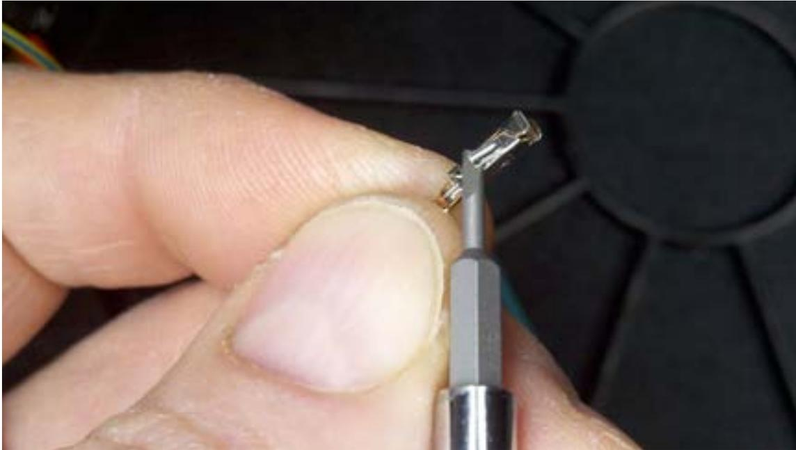
*Using a precision screwdriver to flare the locking tab on a wire terminal from VW OnStar connector*
