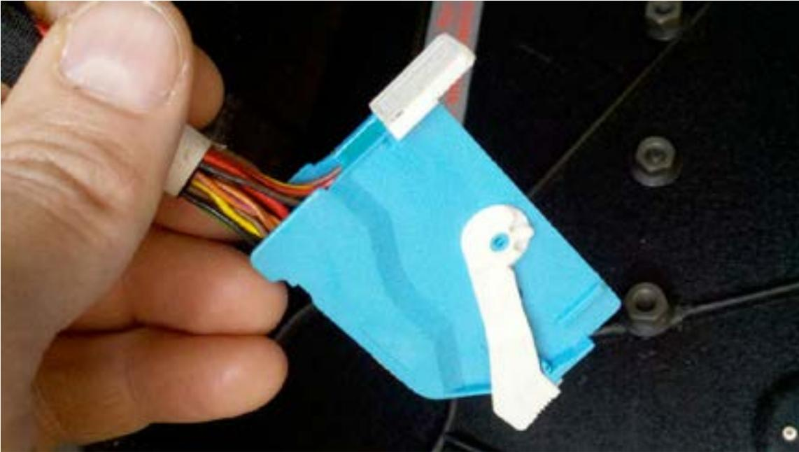
*VW OnStar 42-pin connector outer chassis guard*
