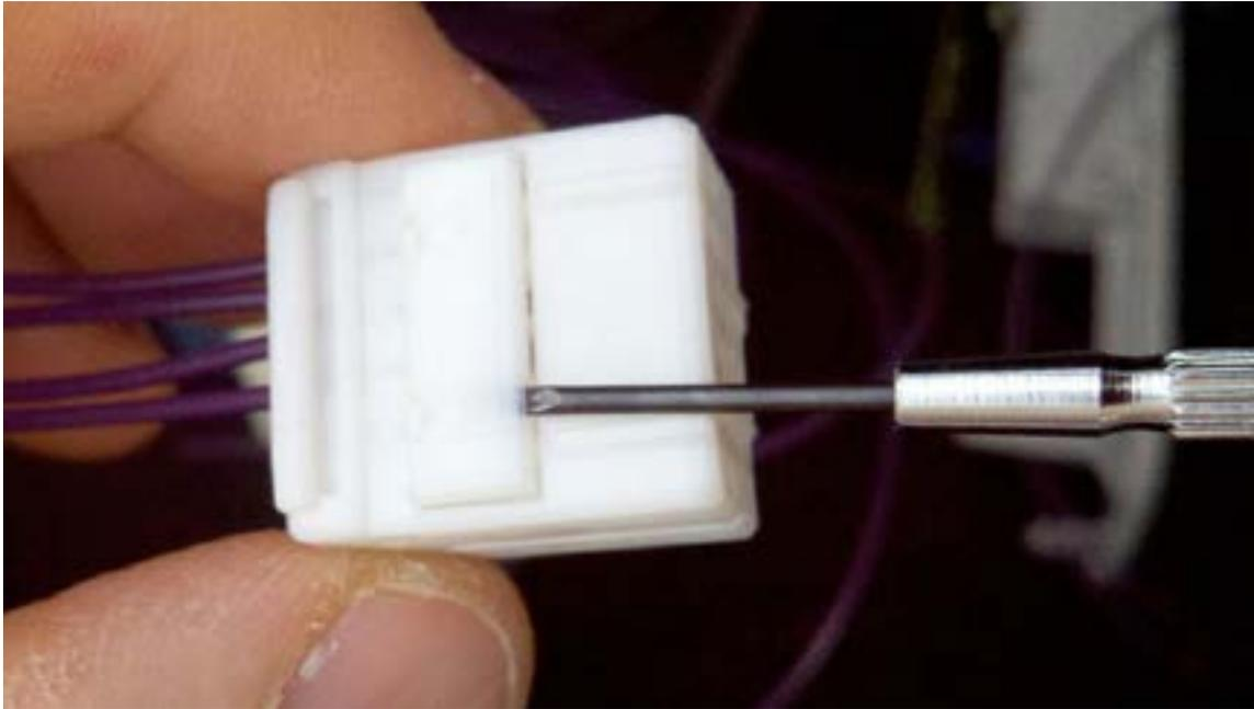
*Releasing the lock on the new 16-pin Bluestar connector (disregard purple wires, they were an early test bundle on my installation only.)*
