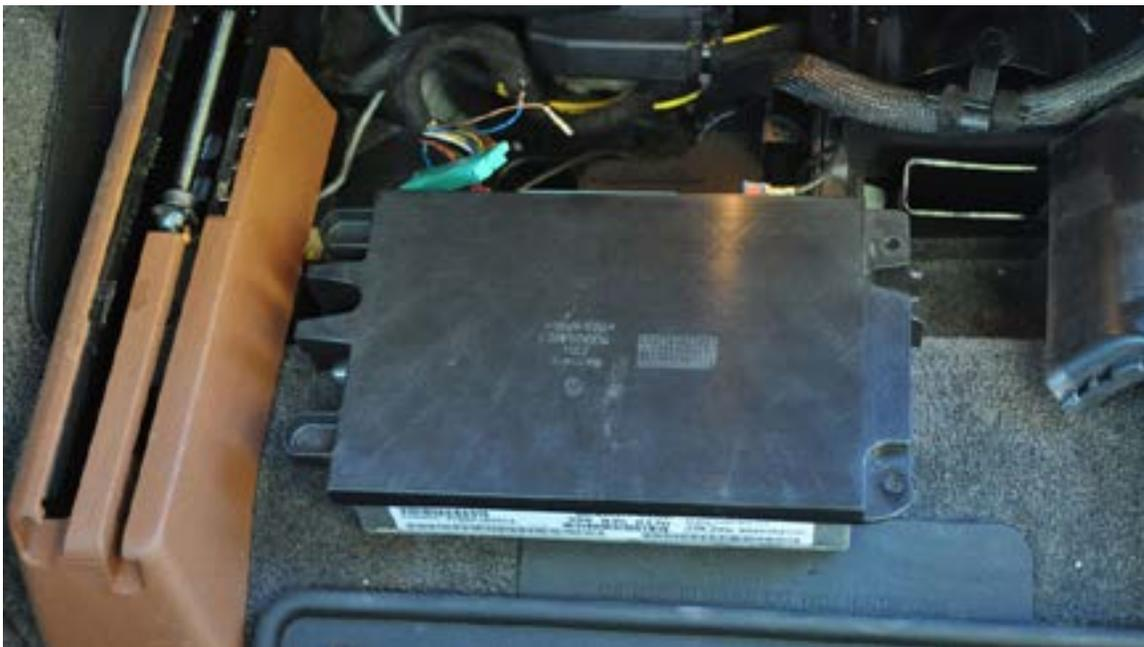
*2004 Touareg OnStar controller mounted in frame under front passenger seat (shown already removed)*
